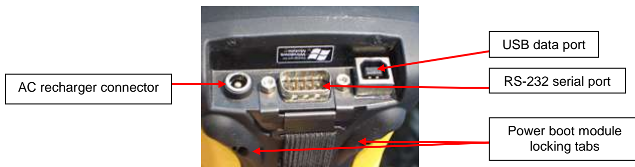
Figure 9: TDS RECON-400 Connectors.
