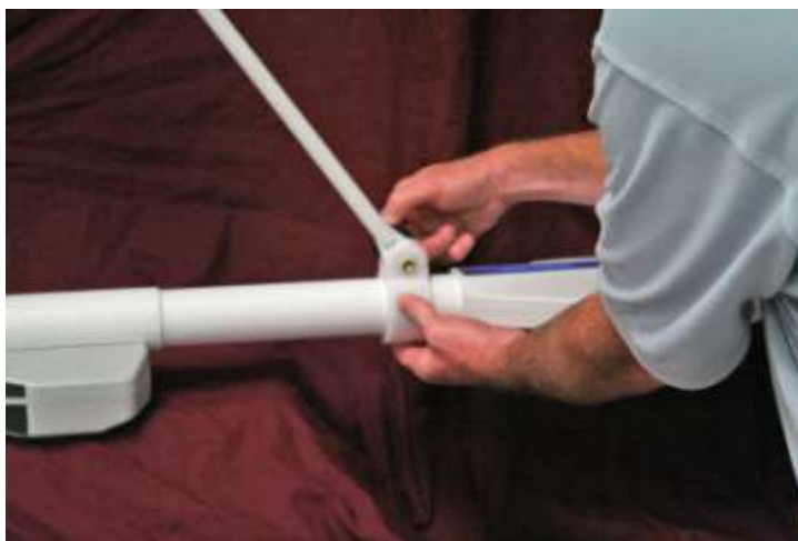
Figure 15: Attaching clamps for low carry handle.
