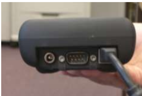
Figure 77: USB “B” connector plugged into PDA USB port.
