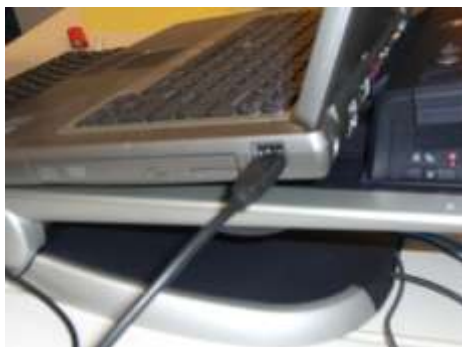
Figure 78: USB “A” connector plugged into free PC USB port.
